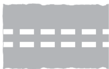
Give way to traffic on major road (can also be used at mini roundabouts)
